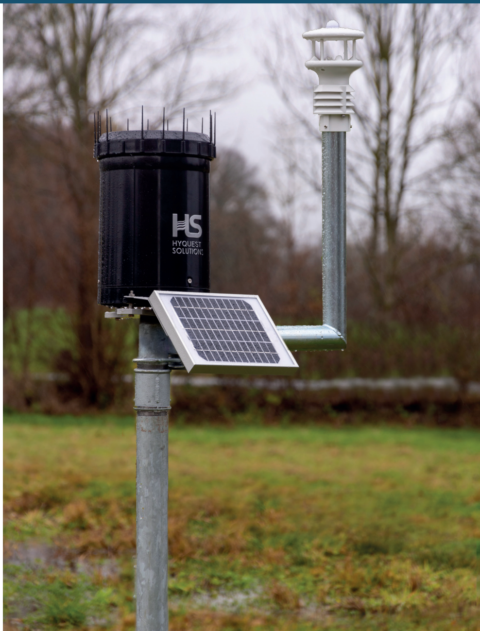
FieldRay Plant Protection - Agrimeteorological Monitoring Station: Rain Gauge with solar panel (left), Weather Station that measures wind speed, solar radiation, temperature, relative humidity, wind direction (right)
