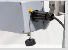
Use the conical cap with a cable. This cap provides a waterproof and dustproof seal for CAT6 RJ45 jacks. Use CAT6 cables with a 7 ... 9 mm/0.28 ... 0.35 in OD or optimal sealing. To install, slide the conical cap onto the CAT6 cable, crimp an RJ45 connector, connect the plug to the RJ45 jack, and screw the cap onto the jack.
