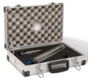
**Portable Field Calibration Device (FCD):** Enables field technicians to run functional tests and calibrations of any given rain gauge in the field
