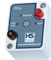
**Pulse Counter CMcbt:** Bluetooth pulse counter providing an interface between the TBRG's reed switch output and the FCD App calibration
