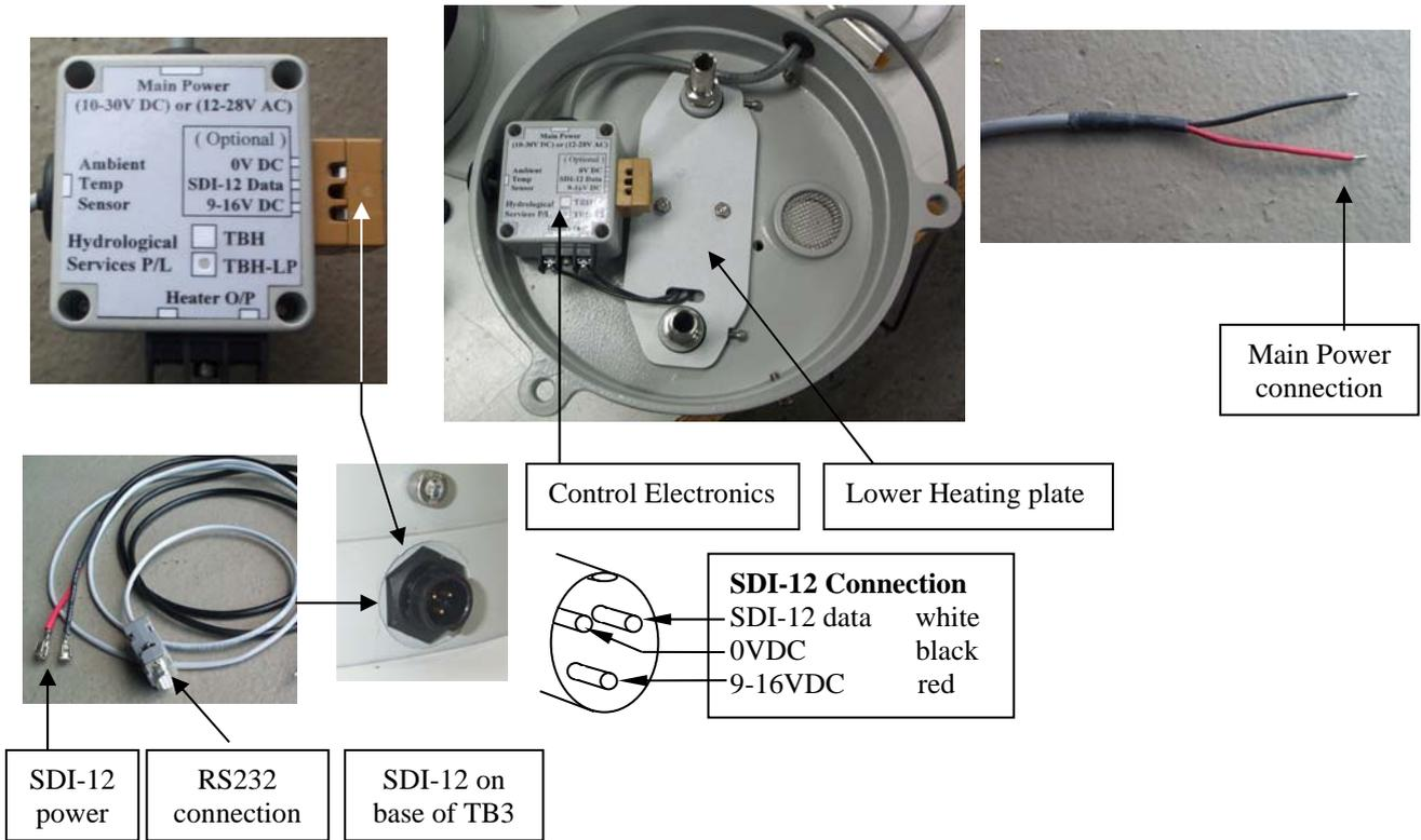
If SDI-12 communications is required, then connect the logger or RTU to the 3 pin connector (Switchcraft brand) on the base of the TB3 rainauge, and supply SDI-12 power.
