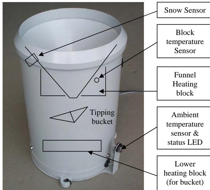
When the TB Heater is “**not Active**” the status LED flashes every 1.5 seconds.
