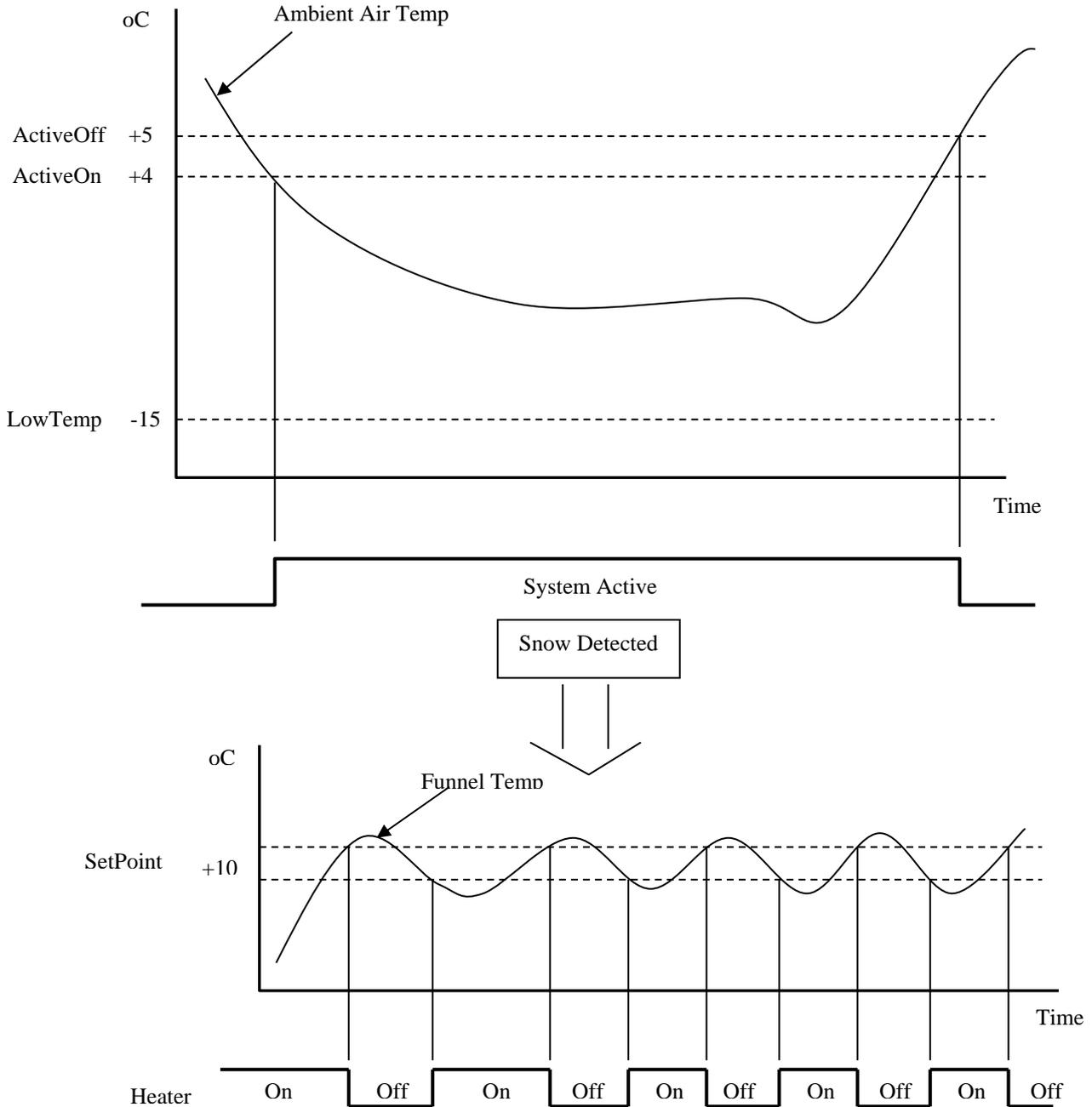
Diagram showing how the “Snow Run-On” timer controls the heater.
