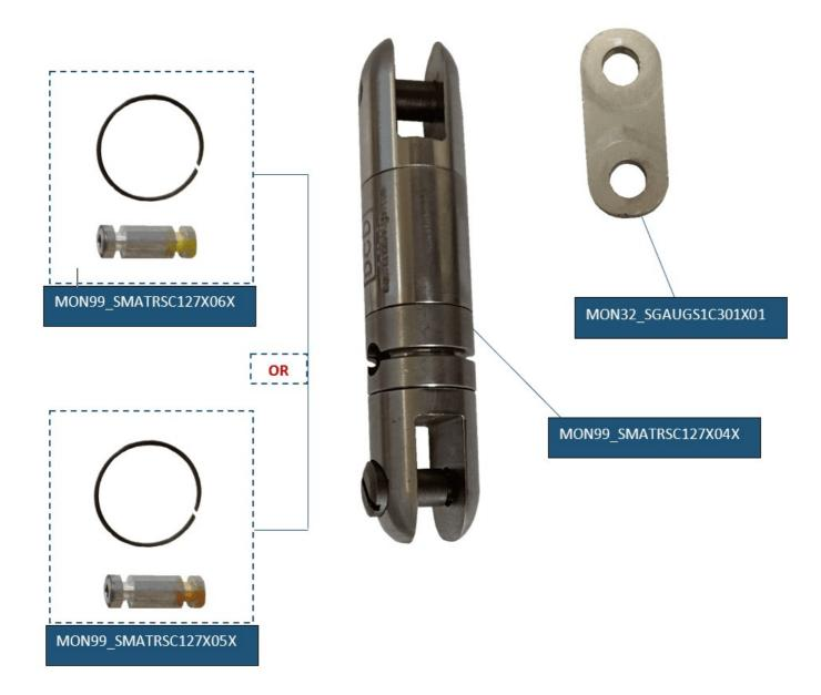
**Note**: The Break-Away kit is supplied with 5 pins and circlips. Either yellow coloured pins for a breaking load of 182 kg or the orange coloured pins for a breaking load of 272 kg.
