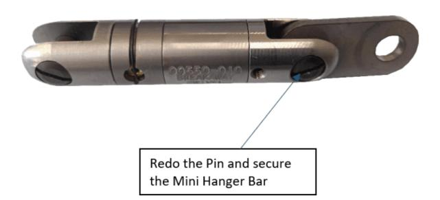
**Note**: The Break-Away Assembly is complete and ready to attach between the C1 connector (Winch) and the Sensor (The Stabilising Weight or Gauging Weight Hanger Bar on the sensor side).
