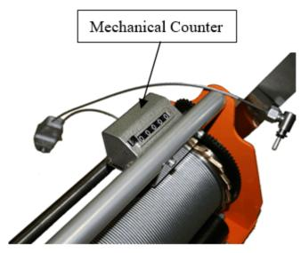
• Lower the current meter and weight to 0.2m, 0.6m or 0.8m of the water level and measure your flow.
