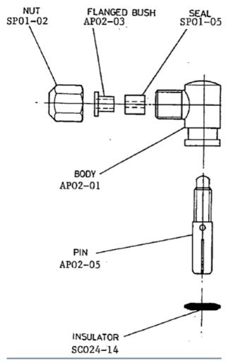
Figure 1 - Angle Plug Assembly AP02
