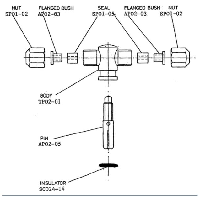
Figure 2 - Angle Plug Assembly TP02
