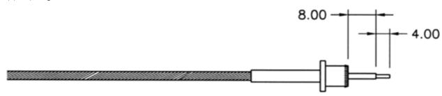
8. Slide rubber seal onto conductor and then push cable into plug. Look into the other end of the plug and check that the conductor wire is in the centre of the plug hole.
