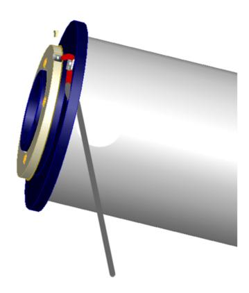
Screw the ring terminal to slipring using the existing screw and tighten the cable clamp and test signal.
