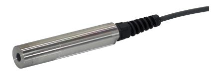
The oxygen sensor uses luminescence-based optical measurement technology and measures reliably and precisely. The low maintenance and small amount of consumable materials needed by the sensor provide immediate returns on investment. Only the membrane cap must be replaced every two years. The sensor can also be used in applications with a very weak water flow. The oxygen sensor is available with a 10-meter or a 2-meter cable.
