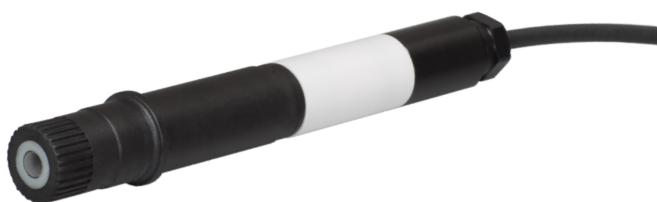
Robust digital pH sensor for operation on TriBox controllers and HS100 DIN G2 rail module. Digital communication ensures safe and trouble-free signal transmission from the sensor to the controller. The high-quality gel pH electrode has a hole diaphragm and is insensitive to dirt, making the sensor ideal for wastewater applications.
